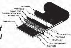
**Bare Steel:** Fabral uses only 29 gauge, <u>80,000 minimum PSI bare steel</u> with a minimum .015 thickness before paint to assure you the thickest, strongest panel in the industry. <u>UP TO 50% STRONGER</u> THAN SOME COMPETITORS 26 GAUGE, 40,000 PSI STEEL.
